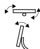
**Step 2**. To adjust the **elevation angle**, loosen the bolt and nut at the bottom of the curved slot. Adjust the angle of the antenna.
